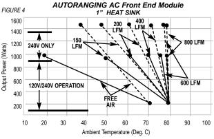
**EXAMPLE:** For your particular application you have determined that you will require an input power of 750 watts with a 120VAC input. Selecting the CASMM1CLXX, will provide you with the 750 watts. This unit is 97% efficient at 120VAC, therefore, the power dissipation from the module will be approximately 22.5 watts. By viewing Figure 3, it can be determined that in a 60 °C environment, forced air cooling of 200LFM with a 1/2" heat sink will be required.
